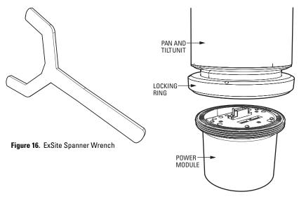
Figure 17. Removing the ExSite Pan and Tilt Unit
